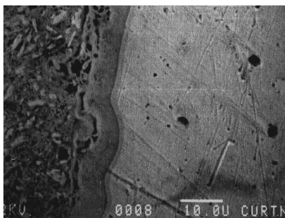
Figure 2. SEM backscattered electron micrograph of a polished cross-section of a positive lead/acid battery plate.
