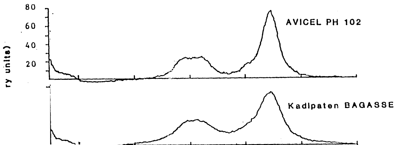
Figure 3 : X - ray diffraction pattern of AVICEL PH102 and MCC made of Kadipaten Bagasse
